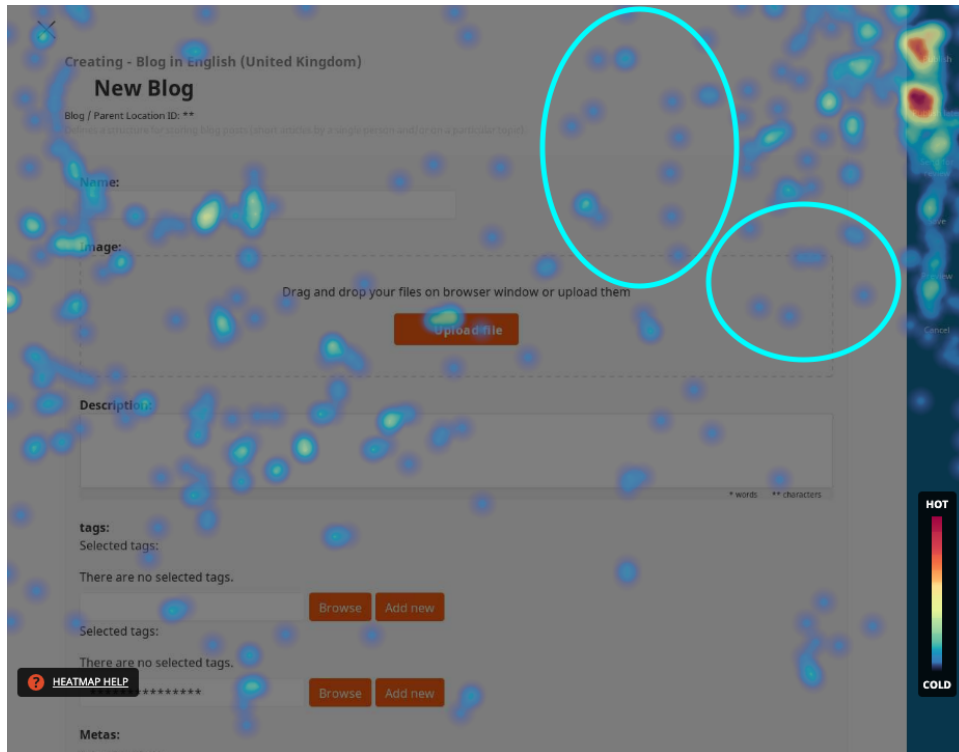
Screenshot 6. View of user testing heatmap, showing extra clicks made when displaying and closing dropdown menus included in grouped buttons (circles added).
